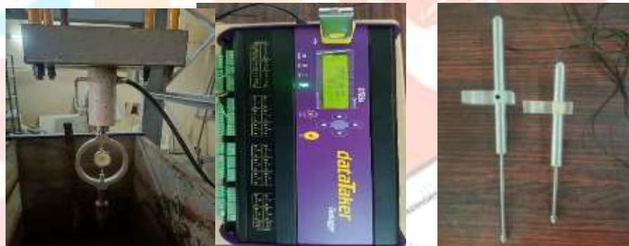
Fig 1. Testing tank with loading frame, Data Taker, LVDTs
