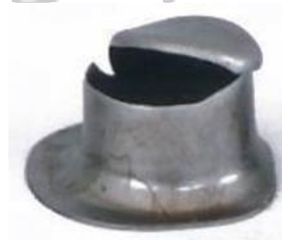
Fig. 3 Fracture in deep drawing [4]
