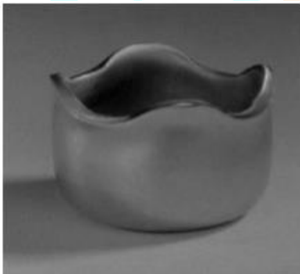
Fig. 5.Earing in deep drawing
