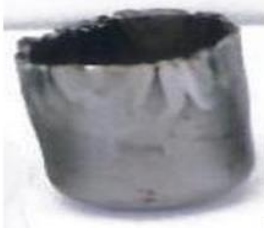
Fig. 4 wrinkling in deep drawing [4]
