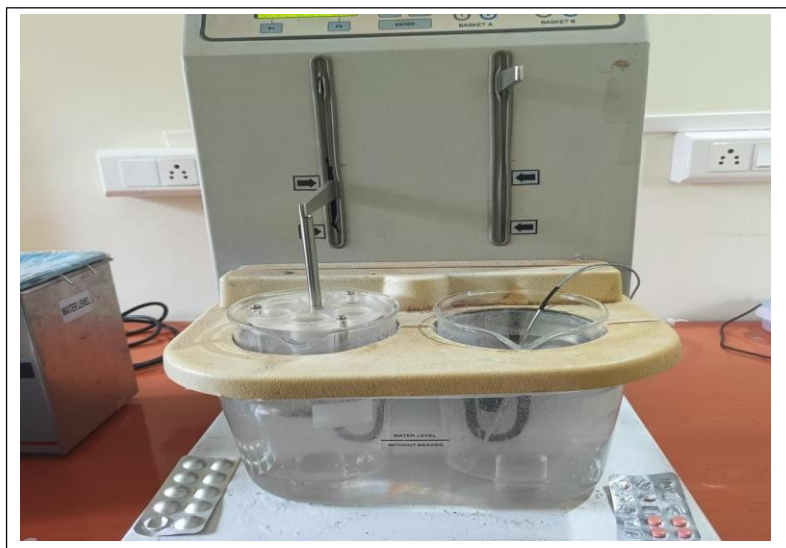
Fig. No. 3 - Disintegration test of Clarithromycin -10 tablet
