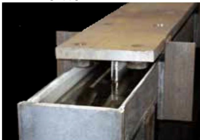
Figure 1.3 Viscous fluid filled between the steel plates
