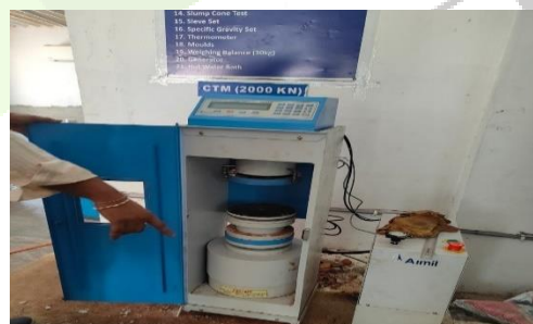
Fig.4.2 Compression and tensile strength testing machine
