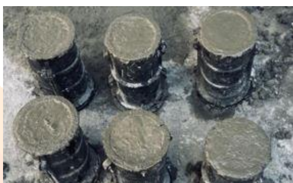
Fig.4.1 casting of moulds
