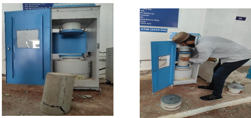
Fig.4.5 splitting tensile strength test on cylindrical specimen
