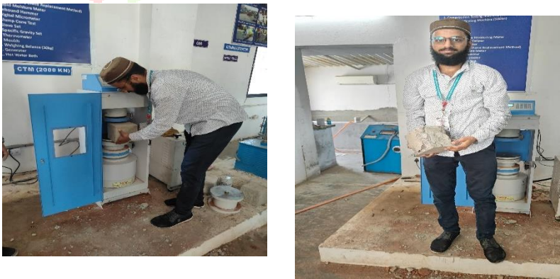
Fig.4.4 compression testing on cube specimen
