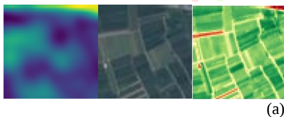
figure 3: sentinel-2 image containing (a) all spectral bands and in .tif format, (b) RGB spectral bands and in .jpg format, and (c) equivalent NDVI converted image in .png format
