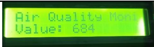
Figure 7.3: Gas sensor analogy values recorded during real-time air quality monitoring.
