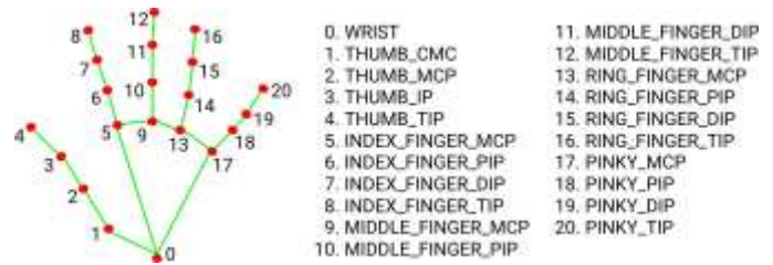
Fig. 6. Mediapipe Hand Landmarker model
