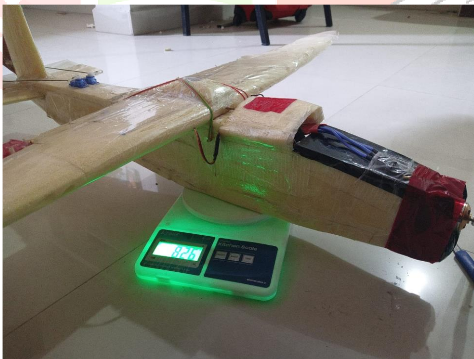
Figure 4 All up weight of RC plane measure on a weighing scale
