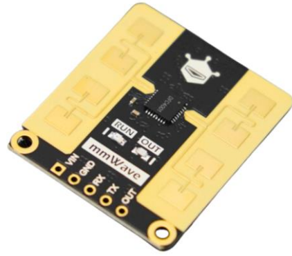
Fig. 5. 24 GHz mmWave radar sensor used for target detection and motion sensing.
