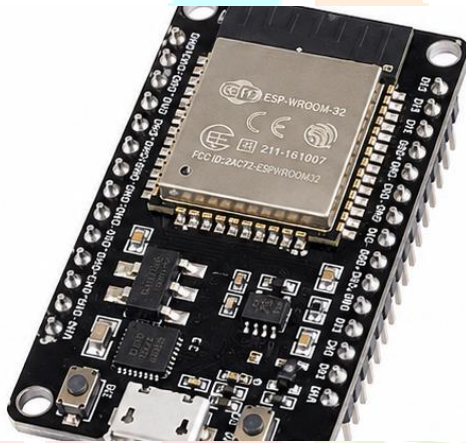
Fig. 2. ESP32 development board used as the main controller of the practical prototype.
