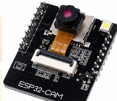
Fig. 3. ESP32-CAM module used for image acquisition and live video streaming.
